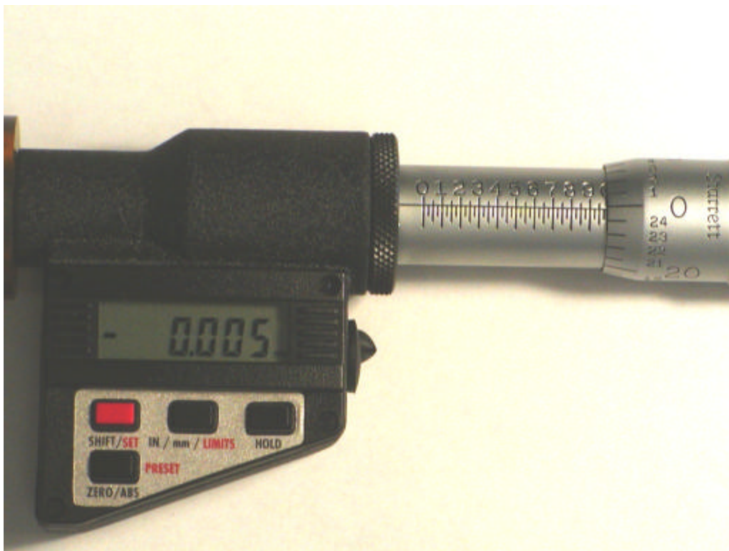
Figure 3. Micrometer Setting for 5 micron depth setting. Note the position of the Micrometer Thimble which is set to the fully retracted position of 1” and indicates the setting of “.0-0”. Note that the digital display shows a value of -0.005 millimeters (5 microns).
